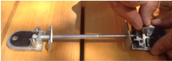
Setting Up Bottom Brackets with bolt, nut, and brackets
