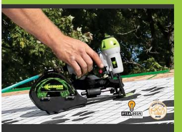
The CN100B is the premier pneumatic cap nailing innovation. When you need to quickly and safely lay down underlayment, this is the tool for you. And with a fastener capacity of 200 caps and nails, reloading is easy and efficient—another time-saver!
