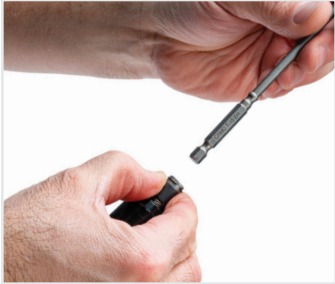
LOAD THE INCLUDED T-15 BIT.
